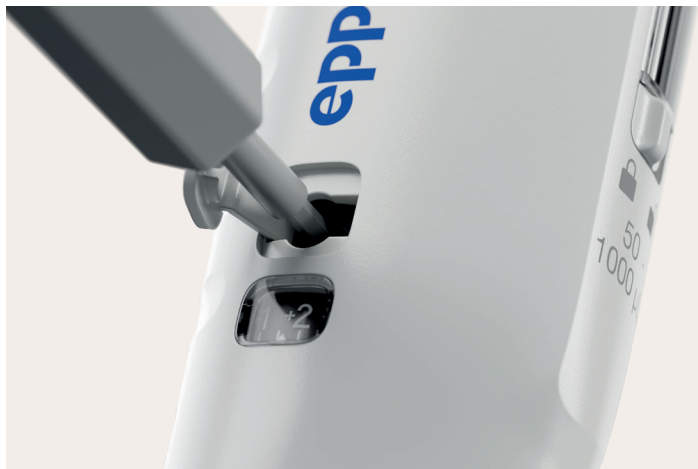
Figure 6: Illustration of the temporary adjustment opening on the Research 3 neo , featuring the window below that displays numerical indicators of any adjustments made. The provided tool is shown inserted into the adjustment opening, enabling changes to the temporary settings. Returning the indicator to zero restores the pipette to its factory calibration settings.
